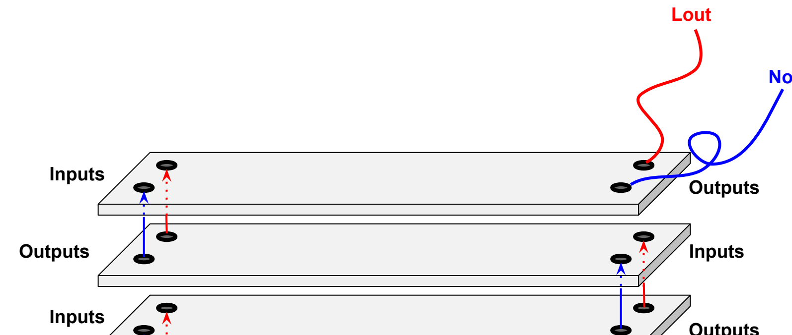
Figure 4: Odd number of FW modules per stack: Inputs and outputs wind up on opposite sides of the stack.
