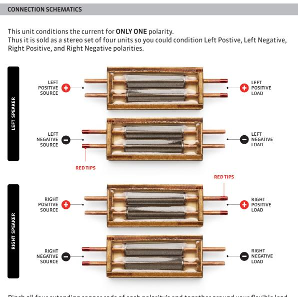
Pinch all four extending copper rods of each polarity's end together around your flexible lead and solder your lead to all four ends simultaneously. This is 16mm<sup>2</sup>, a large iron is recommended. (We use 150 Watts.) Simply solder over the red markings; they will not interfere. Use ample flux. This copper is highly treated. Oxides are normal and per design. Arrow on the side always points towards the red markings.
